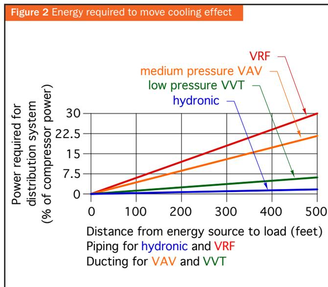
*Figure 2* compares the energy required to move the cooling effect through a building. It assumes that the thermal energy is supplied by a vapour/compression source such as used in a VRF/VRV system. The vertical axis represents the percentage of the compressor power required to move (not create) the cooling effect generated by the refrigeration system. The horizontal axis represents the distance from the thermal energy source (e.g., boiler, outdoor unit, etc.) to the load.
