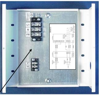
Remote mount box base with removable electrical panel and harness wiring diagram
